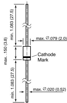
Dimensions are in inches and (millimeters)
