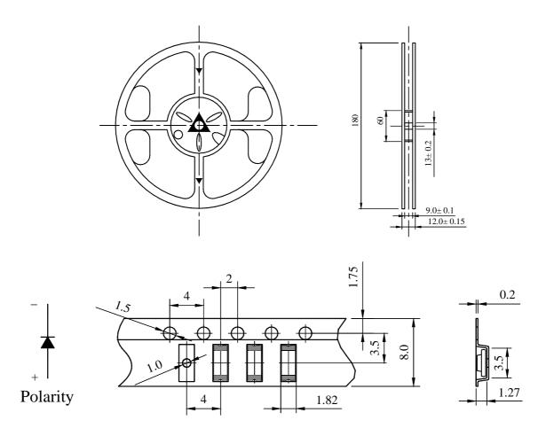
Reel Lead Min.60mm No LEDs
