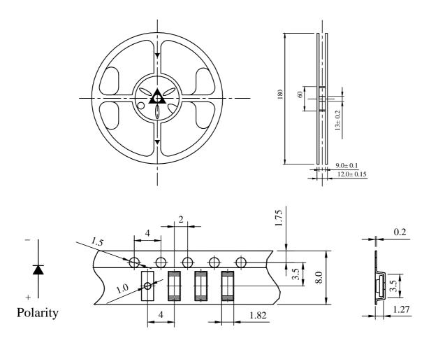
Reel Lead Min.60mm No LEDs
